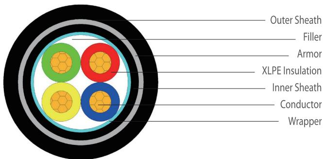
**Rated voltage: 0.6/1kV-four core**
