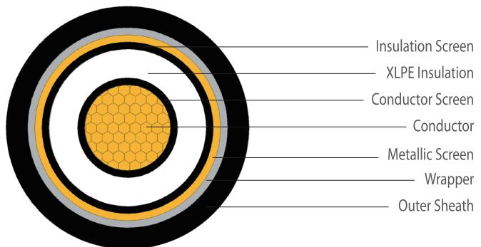
**Rated voltage: 3.6/6kV -single core**
