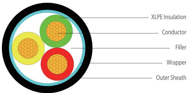
**Rated voltage: 0.6/1kV-three core**
