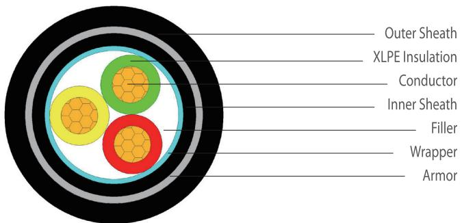
**Rated voltage: 0.6/1kV-three core**
