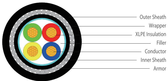
**Rated voltage: 0.6/1kV-four core**
