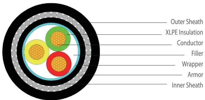
**Rated voltage: 0.6/1kV-three core**
