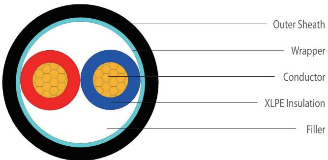
**Rated voltage: 0.6/1kV-two core**
