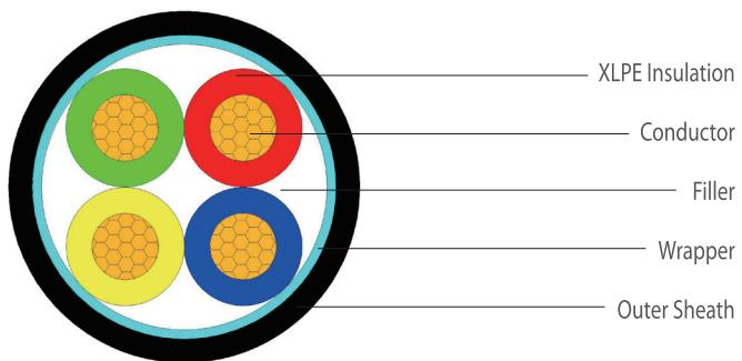
**Rated voltage: 0.6/1kV-four core**
