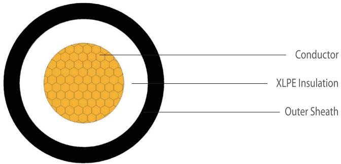
**Rated voltage: 0.6/1kV-single core**
