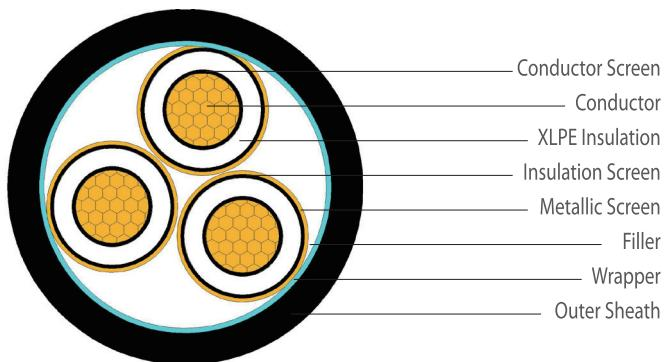
**Rated voltage: 3.6/6kV-three core**
