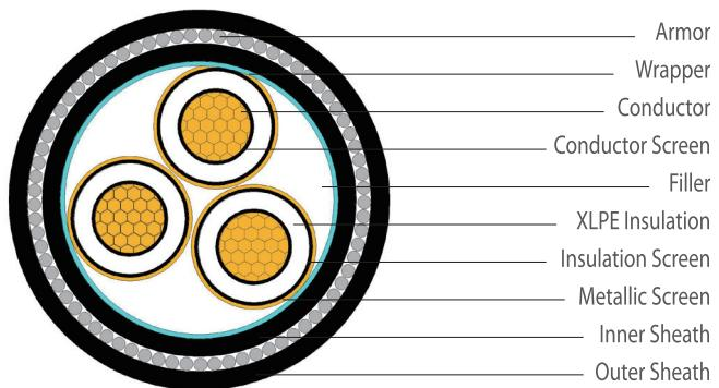
**Rated voltage: 3.6/6kV-three core**
