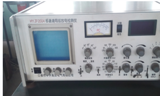
Multi-channel partial discharge
