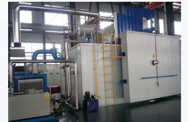
HS.VDR-10 II Vacuum filling equipment
