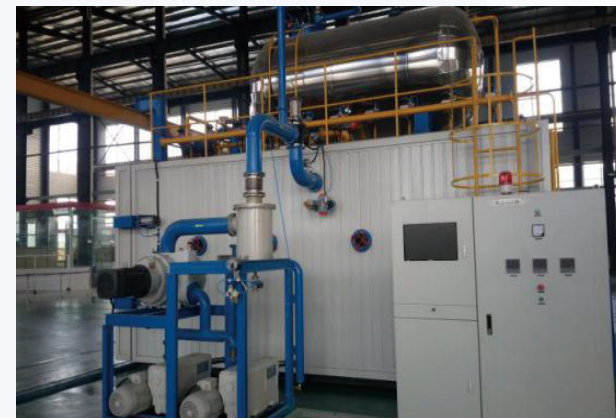
HS.VDH-35 II Vacuum drying equipment
